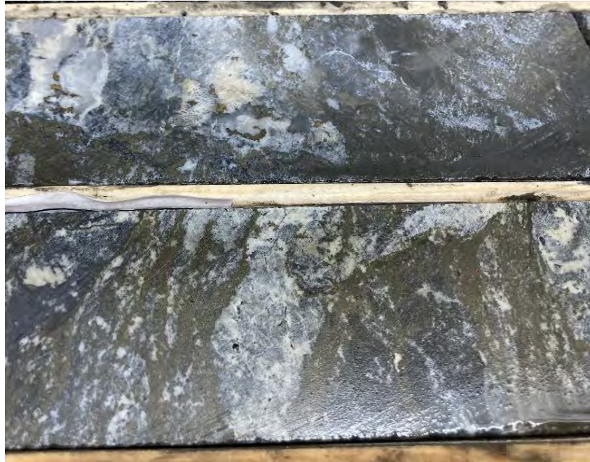
Figure 7.8 – Hydrothermal Breccia Containing Fragmented Massive Sulphides and Carbonate Host Rocks Cut by Quartz-Carbonate-Chalcopyrite Veins
